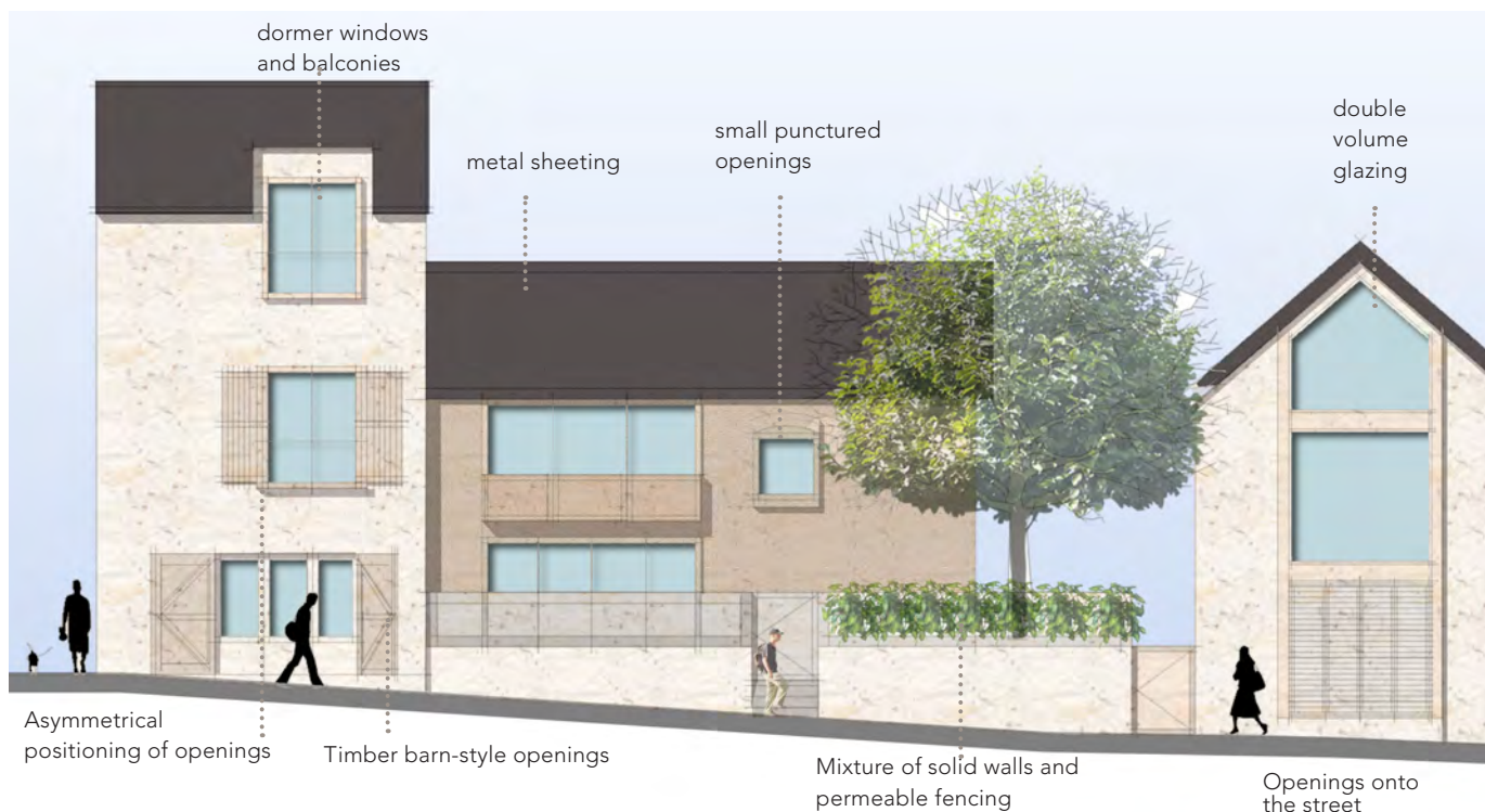
Figure 52. Indicative Elevation along a Rural Hamlet Road
